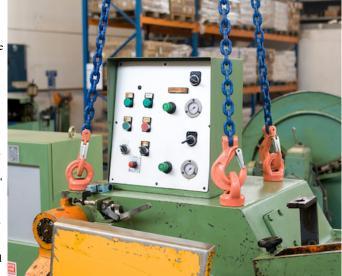
"Using the right swivel hoist ring and rotating eyebolt means there is no more second-guessing the reduced working load limit of a standard eyebolt because it is not an inline pull. The load limit is easily checked as it's forged into the product and doesn't change," added Peter.
