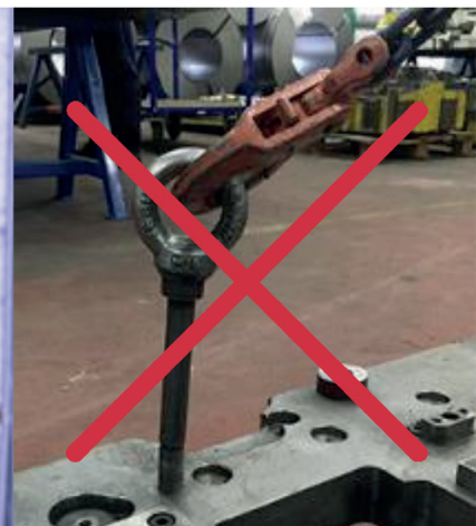
Shouldered Eyebolt Full load rating only at vertical pull
