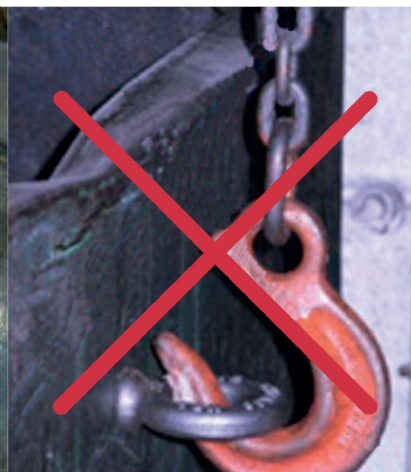
Shouldered Eyebolt Full load rating only at vertical pull
